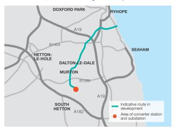
The cables will then run underground for approx. 10km to a new converter station at land South of Murton. A converter station converts electricity between Alternating Current (AC) and Direct Current (DC). AC is used in each country's transmission system, while DC is used for sending electricity long distances.
