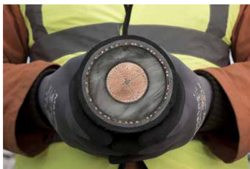
What the cable looks like.
